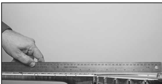
Measuring the bridge placement.
